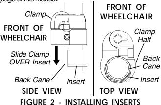
Installing/Removing the Lateral Supports
